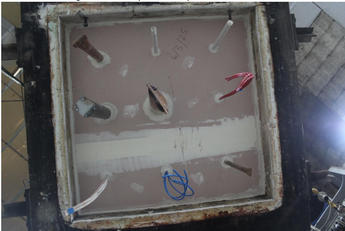
Figure 2 - Exposed face prior to test commencement
